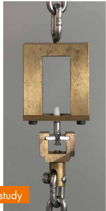
Image*: Test setup – tensile strength test (crosshead speed of 2 mm/min)
